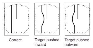
Improper and correct sweep timing
